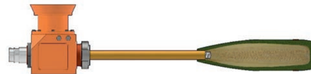
Final position (end) of screw extrusion filling
